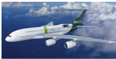
A rendering of Airbus's planned A380 hydrogen-powered flight demonstrator shows placement of a modified GE Passport turbofan on the upper fuselage near the tail of the airplane. Credit: Airbus
