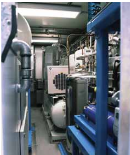
Containerized, high purity (99.5%) aviator grade and human medical liquid oxygen (LOX) system, designed and developed by AFCryo. Credit: AFCryo
