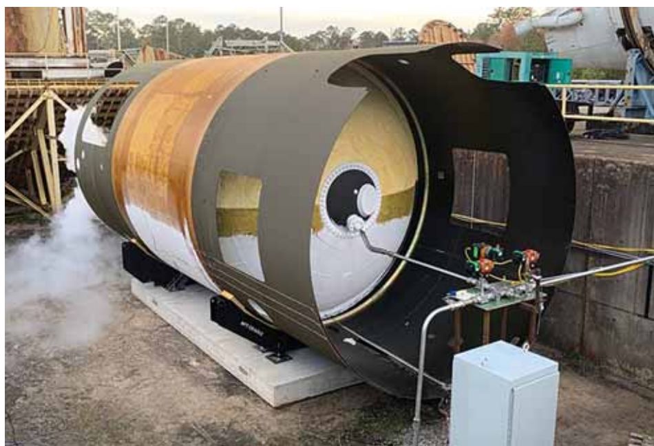
Boeing's all-composite cryogenic fuel tank undergoing pressure testing at NASA's Marshall Space Flight Center. Credit: Boeing
