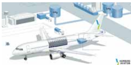
Figure 1. Concept of liquid hydrogen infrastructure for an airport. Credit: Hamburg Aviation
