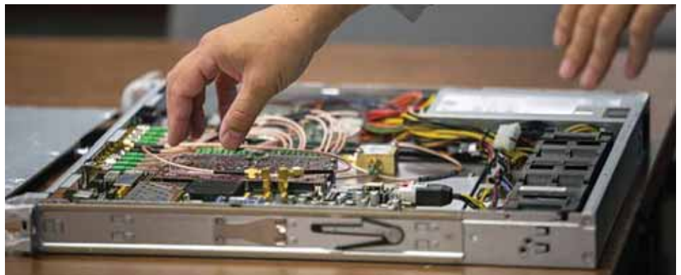
Researchers designed and open sourced a modular field-programmable gate array (FPGA)-based electronics control system. Dubbed QubiC, the system is for superconducting quantum information processors. Credit: Berkeley Lab
